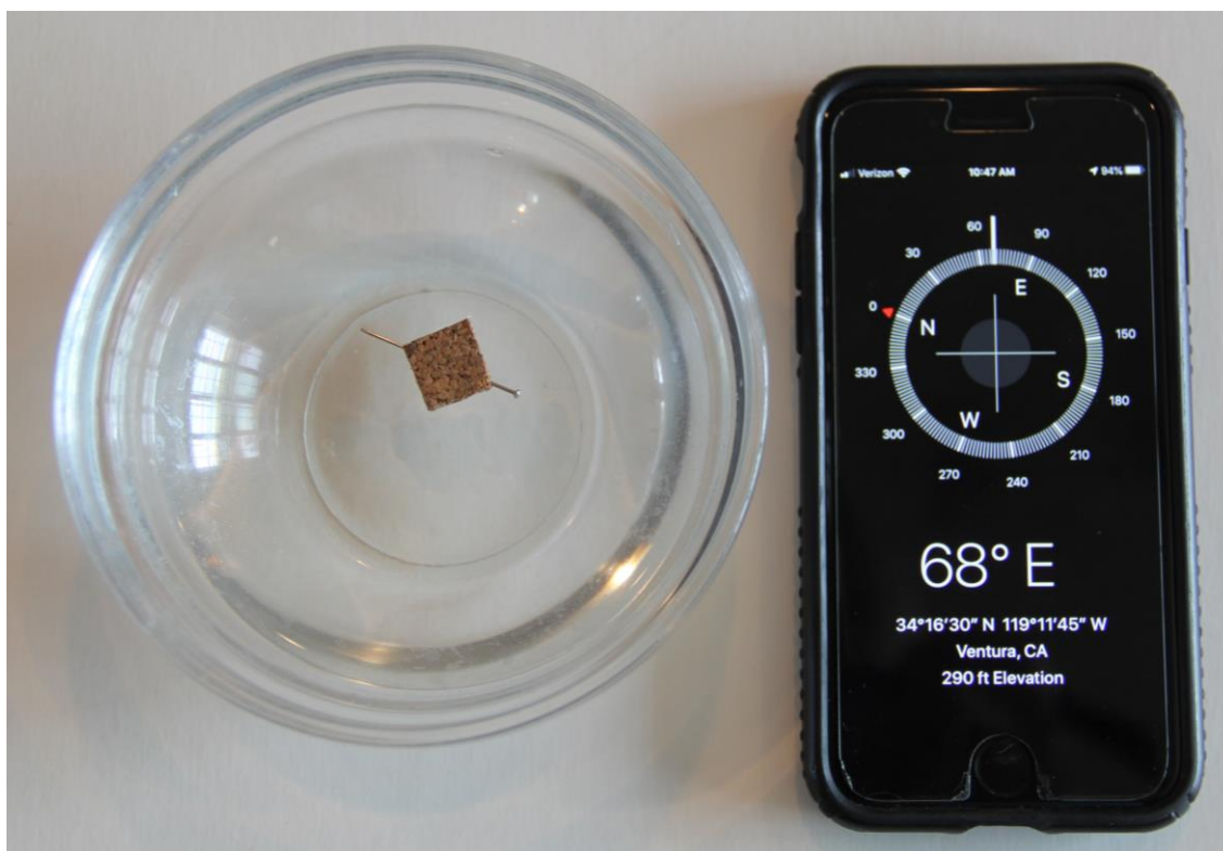
A magnetized steel needle will line up with the needle of a compass to point north.
