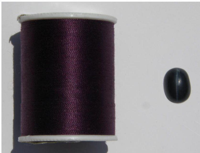
A spool of thread illustrates the cause of “cat’s eye” effect in gemstones.
