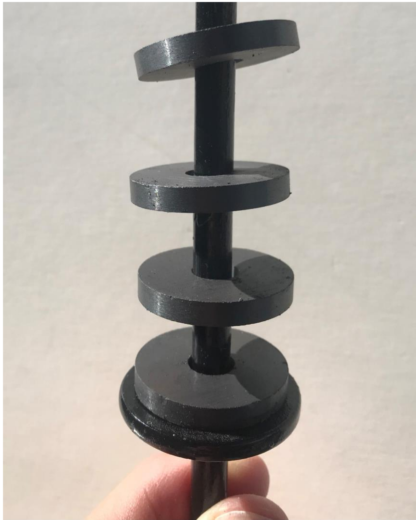
Ring magnets on a stick levitate and bounce in defiance of gravity!
